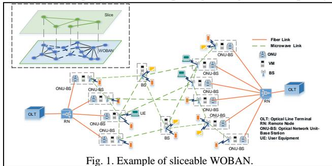
Fig. 1. Example of sliceable WOBAN.
