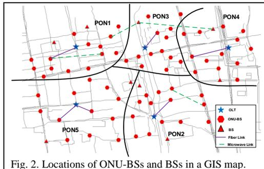
Fig. 2. Locations of ONU-BSSs and BSs in a GIS map.
