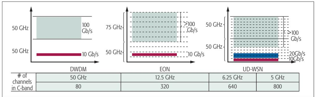
Figure 1. Spectrum usage in the DWDM network, today's EON, and UD-WSN [8].
