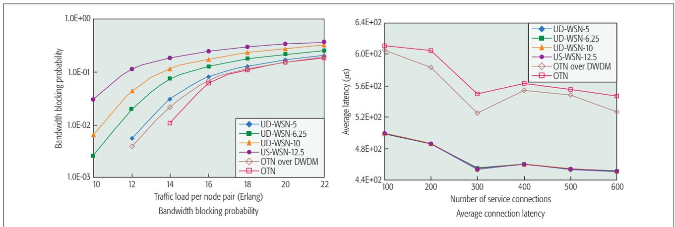
Figure 5. Bandwidth blocking probability and average connection latency.
