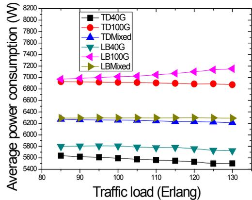
Figure.3 Average power consumption versus traffic load
