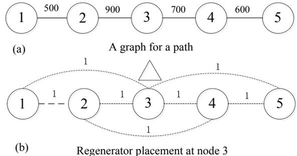
Fig. 2. Example of the regenerator placement at one line rate.
