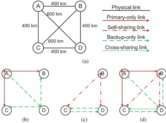
Fig. 1. An example of the shared protection scheme: (a) a four-node fully-mesh network; (b) routing for  $M1 = \langle A; \{B, C\} \rangle$ ; (c) routing for  $M2 = \langle B; \{C, D\} \rangle$ ; and (d) sharing between  $M1$  and  $M2$ .
