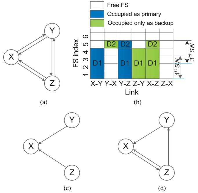
Fig. 2. Illustration for the concepts of SW and SWP: (a) an example network graph; (b) FS usage; (c) a graph  $G_p$  on the first SWP for finding a primary tree for a demand requesting for 3 FSs; (d) a graph  $G_b$  of the first SWP for finding the backup paths for a demand requesting for 3 FSs.
